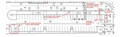
o Concrete curbing along the Fire Lane drive east towards 73rd Avenue will not be removed for new parking.
