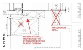
o Concrete curbing at the southwest corner and existing island planter at the east side of the south parking lot will remain and not be removed for new parking spaces.
