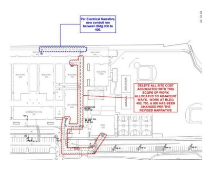
The Electrical Engineer indicated the new electrical feed between Buildings 400 and 900 along the north elevation. To capture this work in Adjacent Ways, the routing was moved to the South
