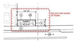
o At Building 100, the existing entry canopy façade enhancements have been reduced. The original design included ACM wall panels which have been changed to MBCI Flexloc 9 ½" wide panels with flush seams. Metal panel wraps at the columns are deleted and will now be painted block. Where light gray vertical
