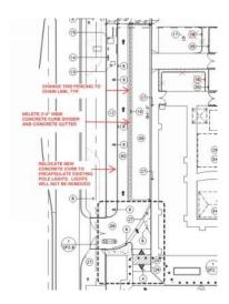
o New concrete curb and drive apron at the widened entry along West Union Hills, secondary entry at the east Fire Lane drive, trash enclosure pad, and new sidewalk west of the existing Service Yard.
